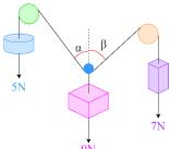
27) The diagram shows three strings, which are tied in a knot K. Two of the strings pass over smooth pulleys and have particles of mass 0.3kg and 0.5 kg attached to them at the ends opposite to K. The other string has a particle of mass m kg attached to it at the end opposite to K. The system is at rest
