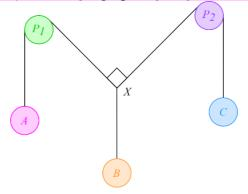
27) Three strings are knotted together at one end, and parcels of weights 5N, 7N, and 9 N are attached to the other ends. The first two strings are placed over smooth horizontal pegs, and the third parcel hangs freely, as shown. The system is in equilibrium. Find the angle which the first 2 strings make with the vertical between the knot and the pegs
