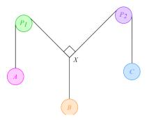
26) Three strings are knotted together at one end, and parcels of weights 5N, 7N, and 9 N are attached to the other ends. The first two strings are placed over smooth horizontal pegs, and the third parcel hangs freely, as shown. The system is in equilibrium. Find the angle which the first 2 strings make with the vertical between the knot and the pegs
